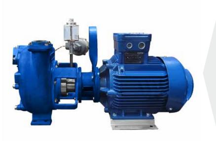
Suction port Threaded - 3" ISO 228 (BSP) Delivery port Threaded - 3" ISO 228 (BSP) Qmax 95 m<sup>3</sup>/h - 1583 l/min (418 USgpm) Hmax 16 m (52 ft) Solids handling 40 mm (1,5") Motor power 4 kW - 5,5 HP Motor type **IEC** standard **Cast iron frame** Motor brand CEMP Weight 144 kg (317 lb)
